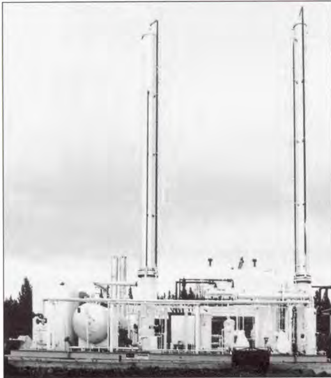
23 USGPM Packaged Amine Sweetening Plant
